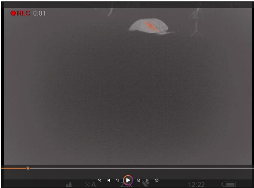
Figure 1. A ‘false thermal image’ of an artificial nest box on 3 rd of March 2024. Orange color indicated a heat source seemingly emitted, for example, by a seal, but lair censuses and camera traps inside lair cavity (Action D2) showed that structure had not been used by seals during the entire season and therefore thermal source was related to the temperature difference between the nest box and the environment.
